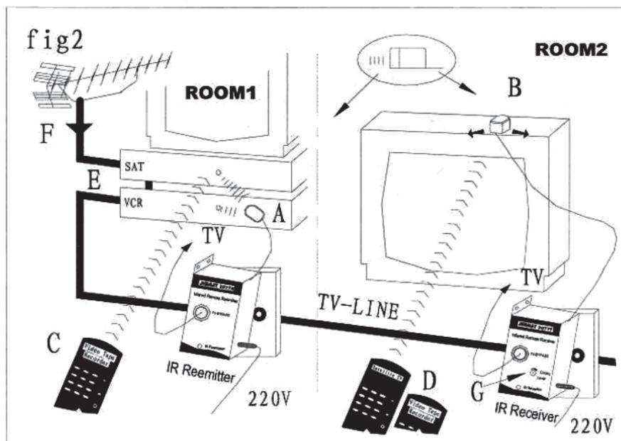
Note: It is convenient to begin this operation with the receiver level to maximum (fig2-G), minimizing later to an operative level without saturations and interferences.
