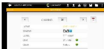
ASuite can monitor specific parameters of DVB-T and DVB-T2 standards such as CNR, CBER or PER, and display them on the application in real time, for each filtered channel.
