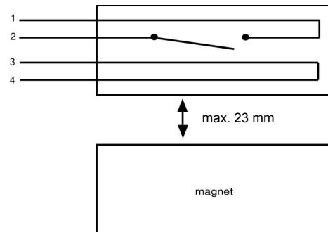
**Surface mounting:** The reed switch or magnet is installed in the surfacing housing. The opening for the lead-in is snapped out of the upper part of the housing where indicated. The fastening screws are covered with the supplied cover caps and with the upper parts of the housing. When mounting on a magnetically conducting surface, anti-magnetic screws and spacing blocks are to be used.
