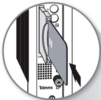
Before turning on the power for the unit, insert the card into the CAM to the bottom, with its contacts towards the left and forward, as can be seen in the figure.
