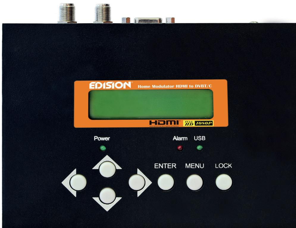
**LCD Display** – It presents the selected menu and the parameter settings. The backlight in the display is on when the power is applied.
